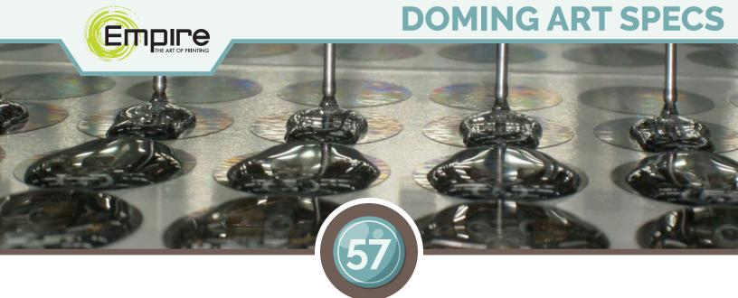
Add dimension and durability to your decals with doming. Doming is a process that creates a lens-like appearance over the part's surface. To achieve this, we flood the decal with doming liquid and let it dry into its final shape. Doming is a unique manufacturing process that requires specific design requirements.
