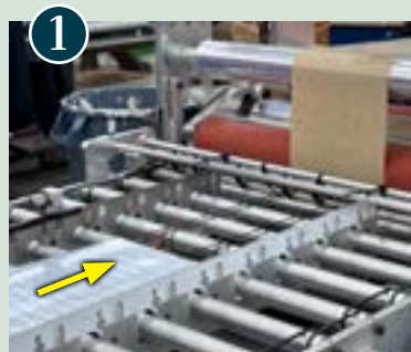
1 sheet is placed on the rollers, directly from the press.
