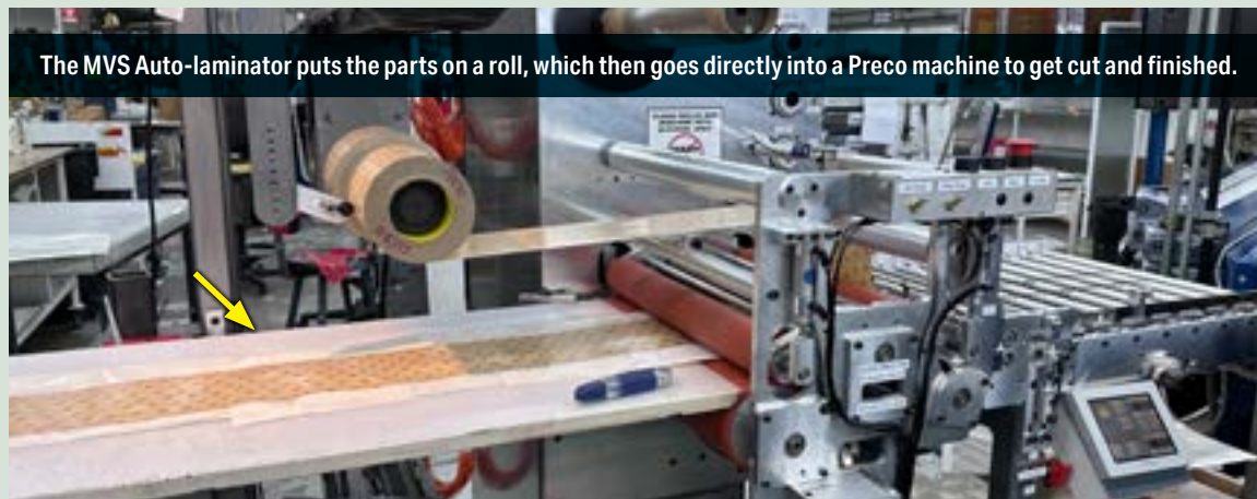
1 sheet is placed on the rollers, directly from the press.
