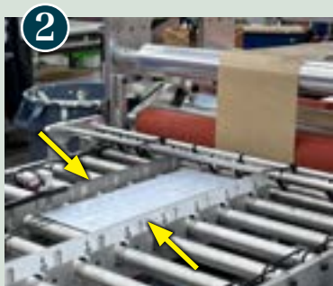
2 Clamps guide the part on the rollers
