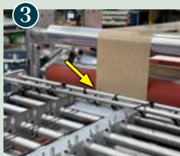
3 The laminator automatically applies lamination / adhesive.
