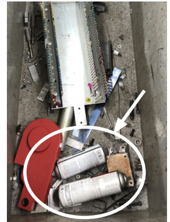
Metal waste and aerosol cans in same disposal bin
